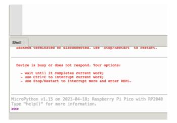
Once it connects successfully, the Shell window should show MicroPython running on the Raspberry Pi Pico.
