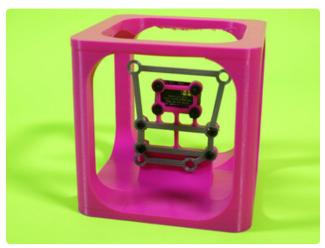
If you are using a mounting plate, mount the plate to the cube using the Metro Mini's mounting holes with M2.5 screws and nuts.
