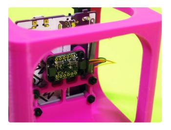
Plug the 9 DoF STEMMA board into the Arduino board using a STEMMA QT cable.
