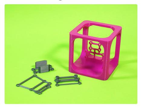
You can use the 9 DoF sensor without an enclosure, but mounting it in an enclosure will give you steadier readings and a better idea of the physical orientation of the sensor. It may be assembled in a 3D printed cube, described below. By default, the cube has mounting holes for a Metro Mini V2. However, there are mounting plates for Metro, Feather and QT Py format boards as well.
