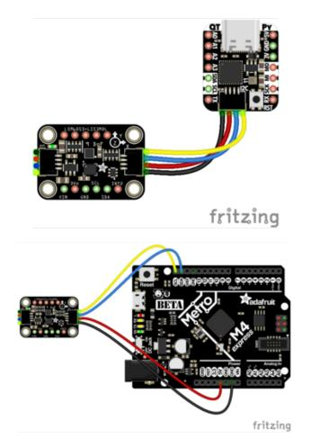
Board 5V to sensor VIN (red wire)
