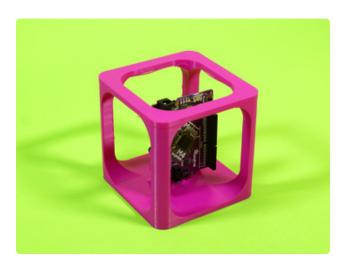
Mount your board using M2.5 screws and nuts.
