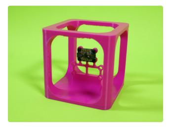
Mount the 9 DoF sensor board to the cube using M2.5 screws and nuts.
